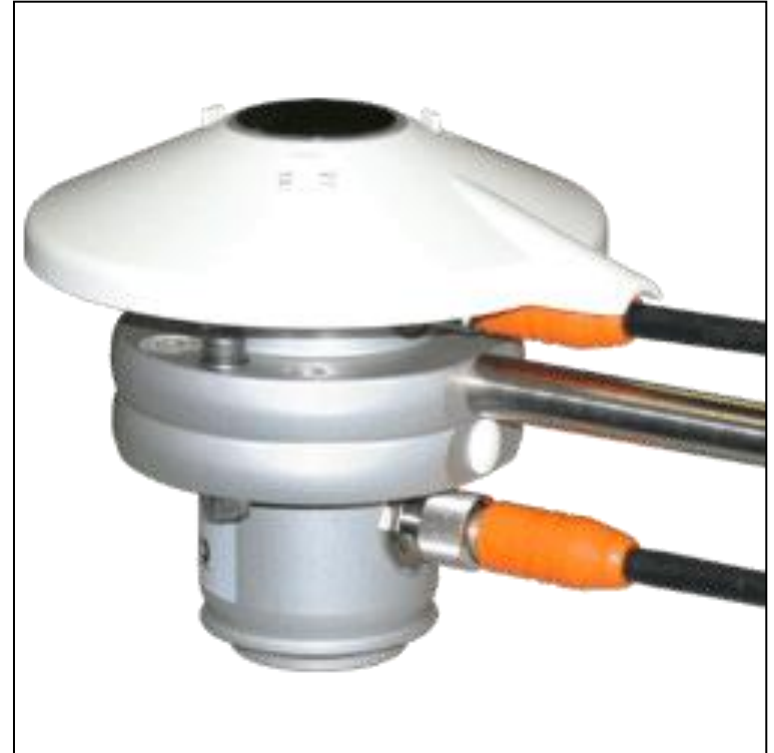
Pyrgeometer – infra red radiation
